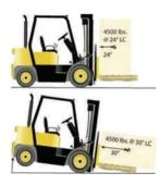
Improperly distributed loads may tip the forklift because the center of gravity has shifted
