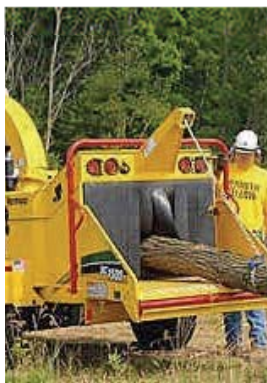
Always stand off to the side of the hopper when feeding materials
