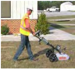
Ground Penetrating Radar
